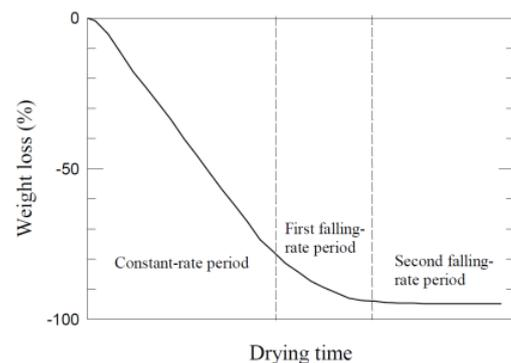
Figure 6 Sludge drying time curve
