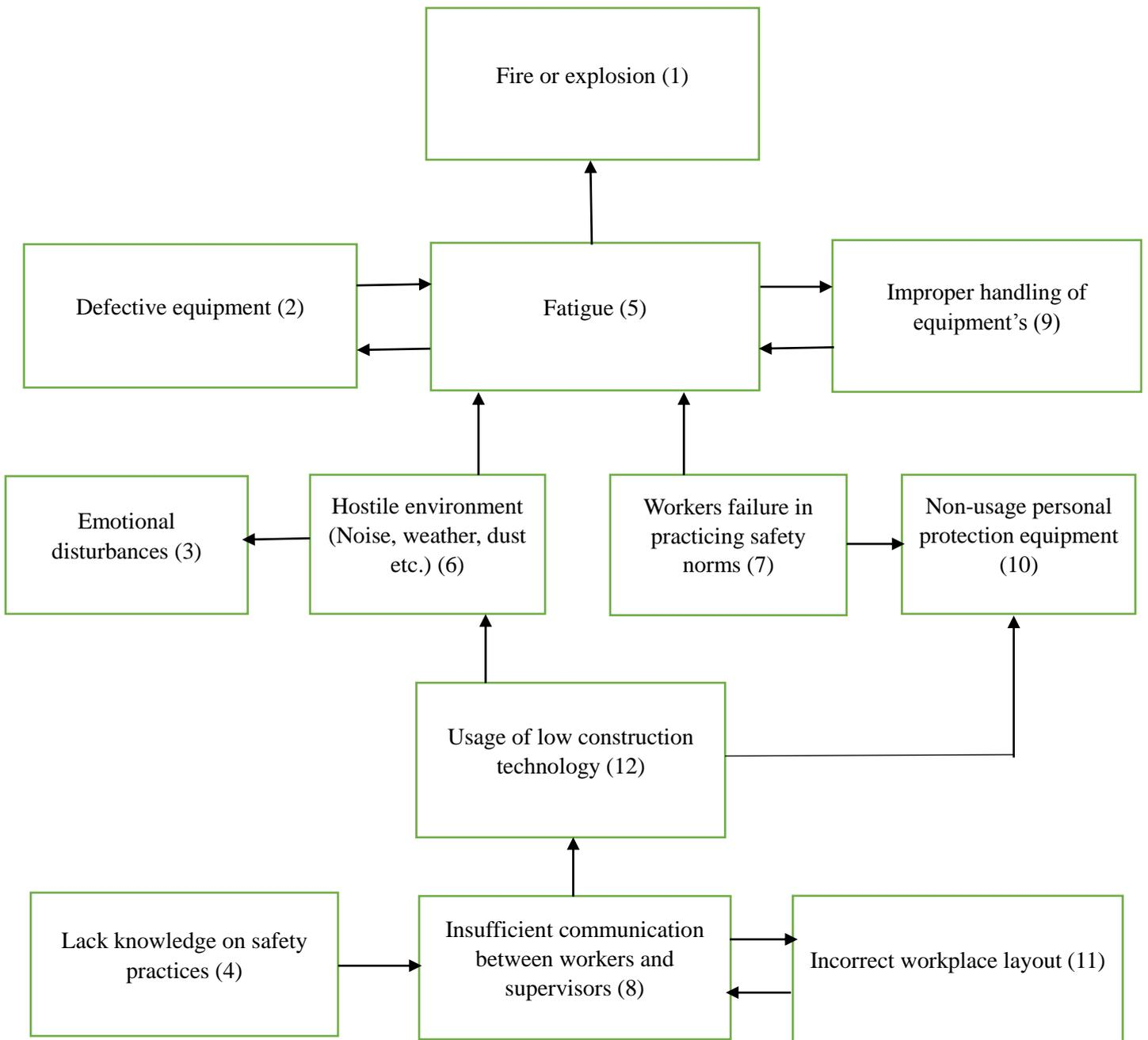
Figure 2: ISM model of factors causing accidents at the construction sites of oil and gas project.
