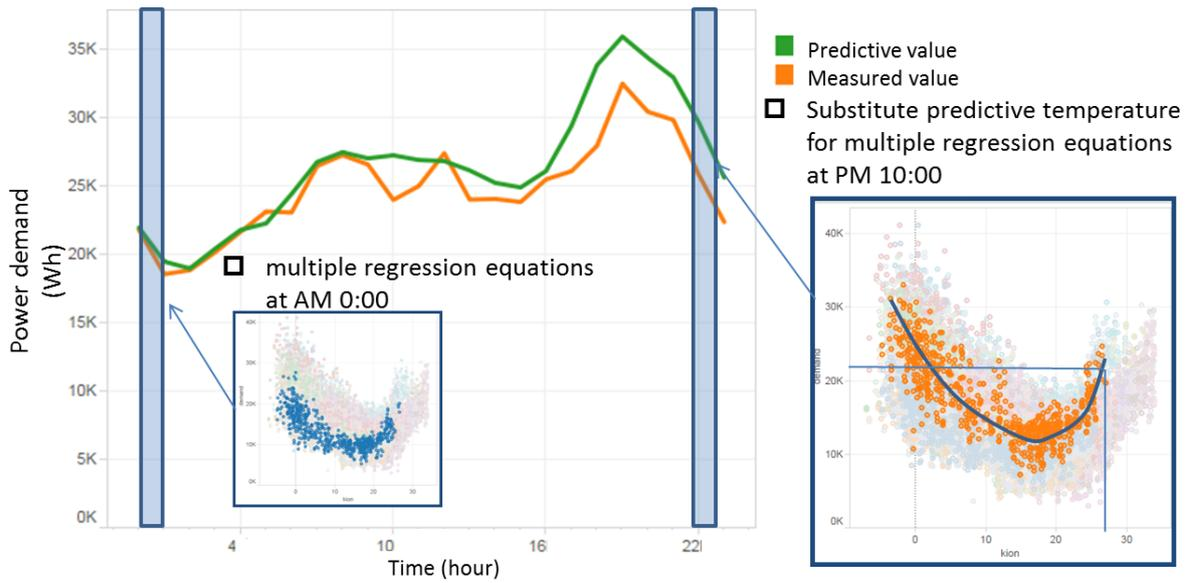
**Figure 3 the schematic chart of 48step method**
