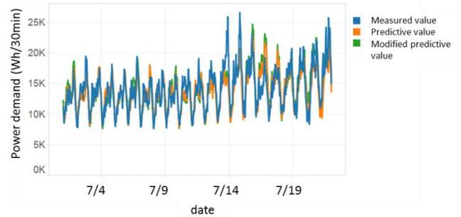
Figure 5 power demands of measured value and predictive value and modified predictive value (Exponential smoothing forecasting)
