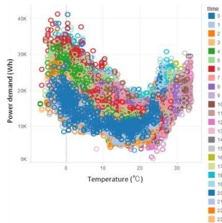
Figure 2 the relationship between power demands and temperatures every hour
