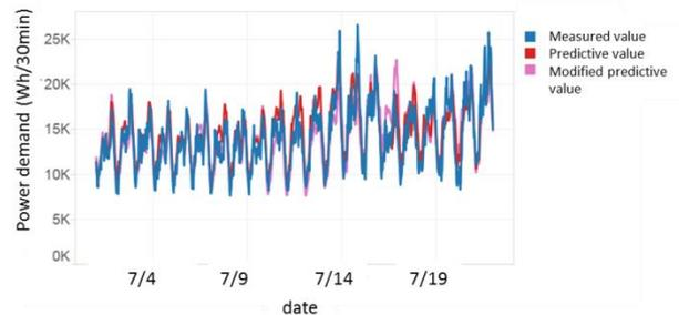
Figure 9 power demands of measured value and predictive value and modified predictive value (step48 method)
