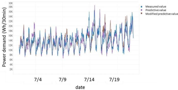
Figure 7 power demands of measured value and predictive value and modified predictive value (ARIMA forecasting method)
