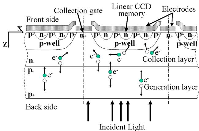
Figure 2: Cross-sectional structure of the image sensor.
