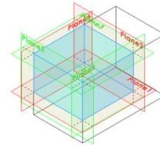
Figure 2. Generated reference planes,  $P$ , which are bounding the TRV.
