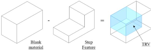
Figure 1. Simple illustration of TRV which is shown as a blue shaded area.
