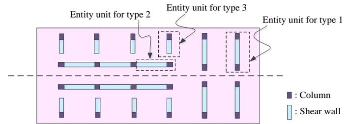
Figure 7: The demonstration of an entity unit in the cast-in-place construction field.
