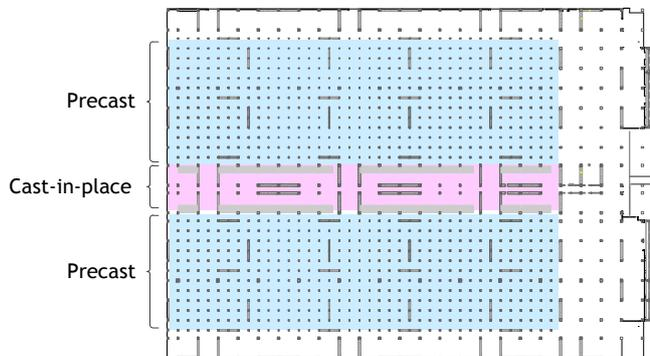
Figure 1: The layout of a precast and cast-in-place construction for a semiconductor fab.
