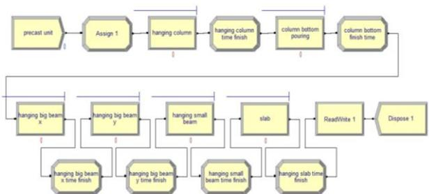
Figure 6: The simulation model of a precast construction process.
