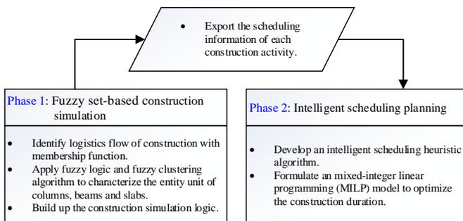
Figure 2: The flow chart of the proposed construction method.
