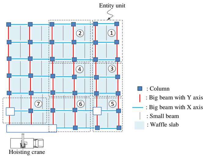
Figure 5: The demonstration of an entity unit in the precast construction field.
