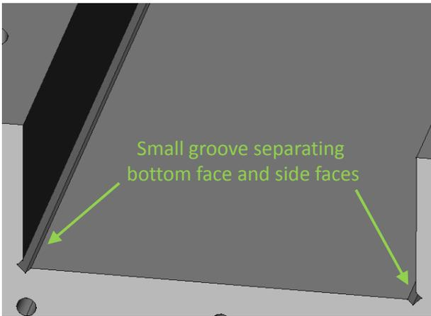
Figure 2: An example of improper slot in solid model
