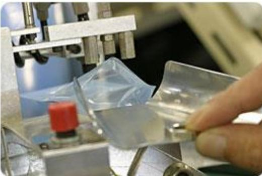
Figure 3: A bagging apparatus of sensor accessories
