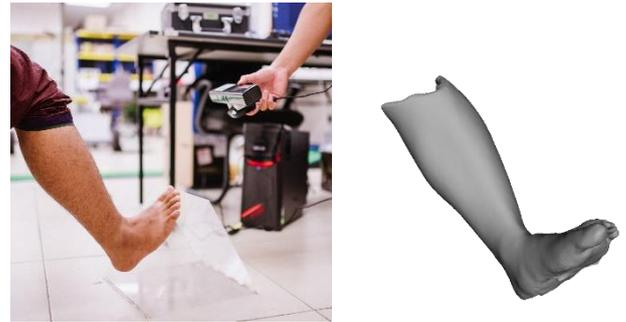
**Figure 2: 3D Scanning process using Microsoft Kinect (Left), Output 3D Limb Geometry (Right)**
