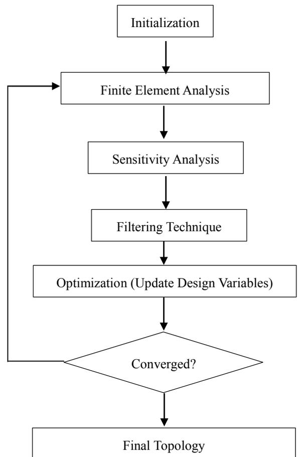
**Figure 7: Workflow of SIMP (Wang, 2007) Algorithm used in this Paper.**
