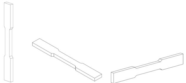
**Figure 5: Specimen Build orientations for Z, X, Y (from left, respectively).**
