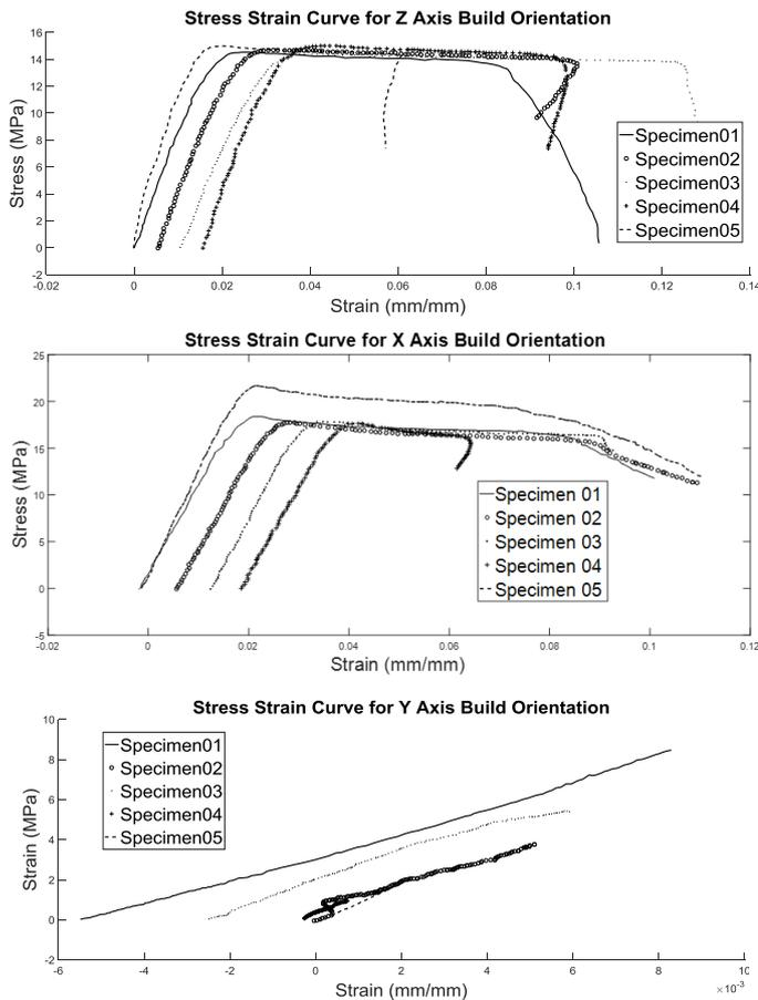
**Figure 4: Engineering Stress Strain Curves for Z-ABS Material for X, Y, Z Orientations (from top) Respectively**
