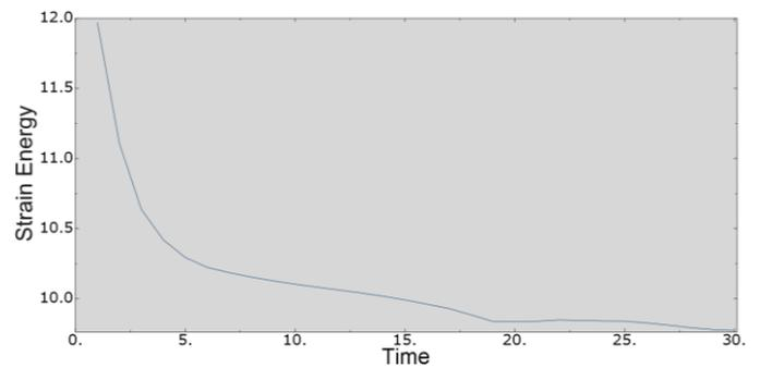
Figure 10: Strain Energy Change against Simulation Time
