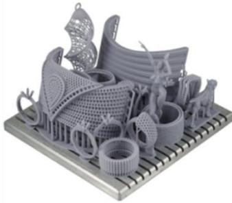
Figure 3: Jewelry master using rapid prototyping machine (Digital Wax 2016).
