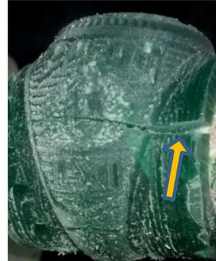
Figure 12: Crack due to over clamped
