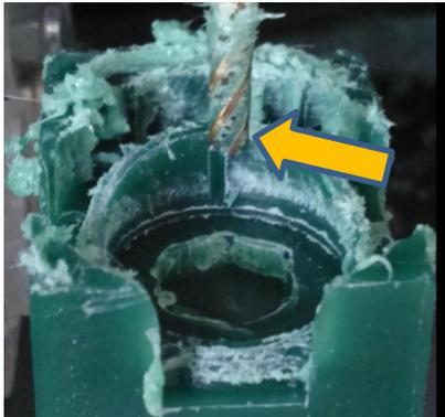
Figure 11: Build-up edge and melting phenomena
