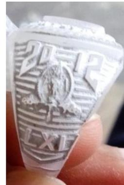
Figure 13: Machining result with resin as material
