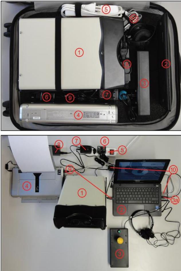
Figure 5: (Upper) The portable screening instrument is fitted and stored in a suitcase. (Lower) The graphical installation guide of the system setup.
