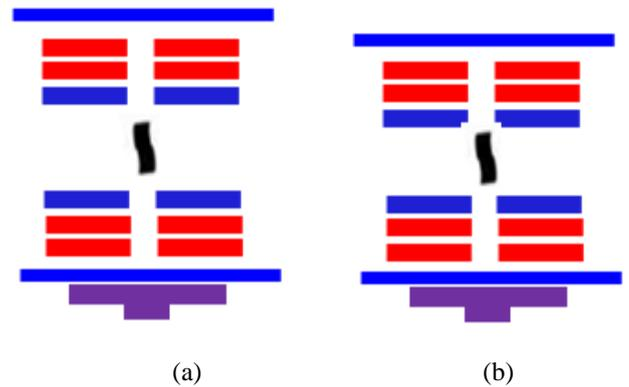
Figure 3: The illustration of the number of product boards per stack, (a) 15 layers (b) 12 layers.
