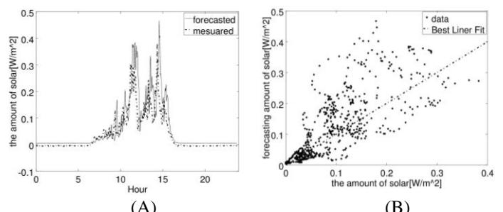
Figure10: Forecast amount of solar radiation after 15 minutes on 2014/10/5.
