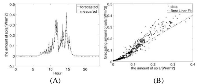
Figure9: Forecast amount of solar radiation after 3 minutes on 2014/10/5
