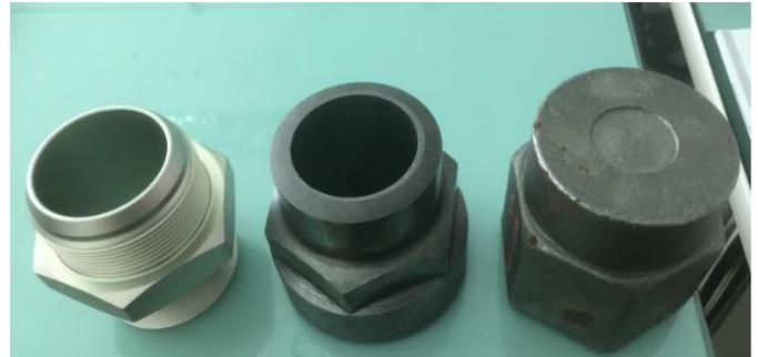
Figure 2: Product photos (cold forging, hot forging).
