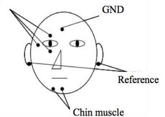
Figure 3.2.2: Electrode of face
