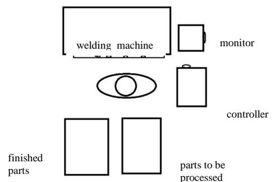
Figure 1: Layout of workstation 1.
