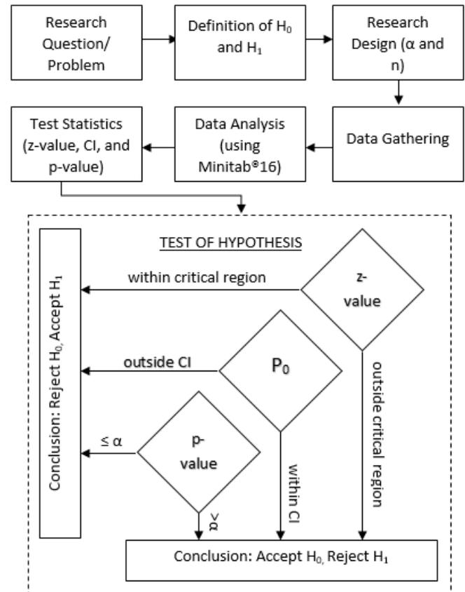
Figure 1: Proportion of One Sample Test of Hypothesis Flow Chart
