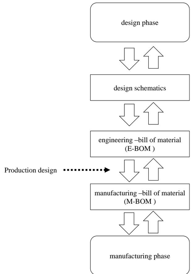
Figure 2: Flow of information from design phase to manufacturing phase
