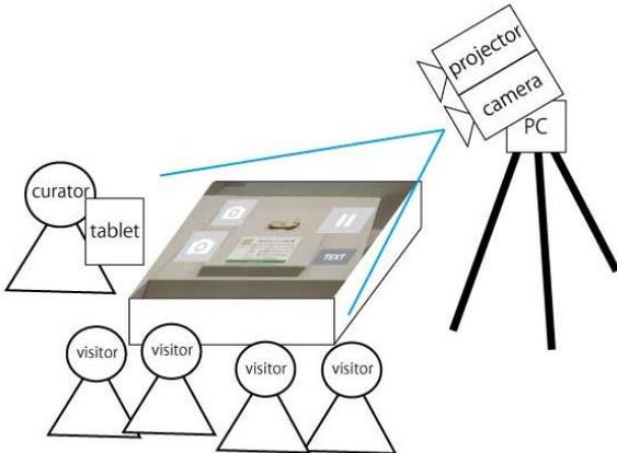
Fig.1. Example usage of this system
