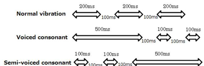
Figure 6: Timing of vibration
