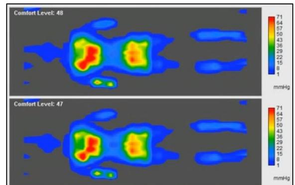
Figure 4: Example of sleeping body pressure data (Vista Medical Ltd. (2016)).
