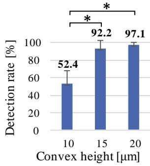
Figure 3: Detection rate for each convex height of defect
