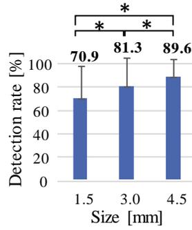
Figure 4: Detection rate for each size of defect
