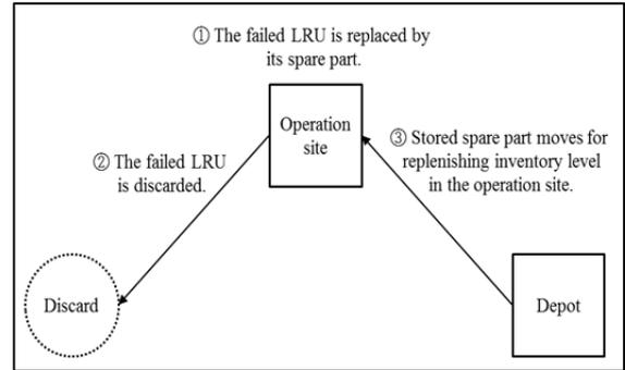
Figure 2: The replacement procedure of failed LRU
