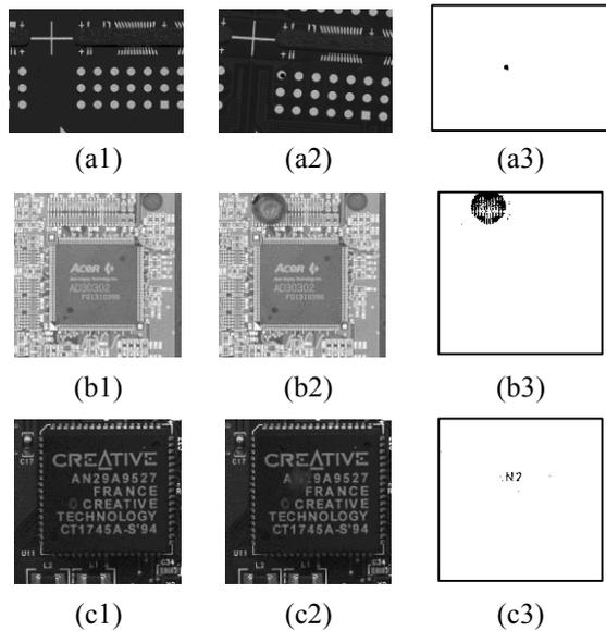
Figure 3. E-M position and image subtraction for PCB defect detection: (a1)-(c1) PCB templates; (a2)-(c2) test PCBs; (a3)-(c3) defect detection results.
