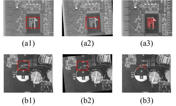
Figure 2. Performance evaluation of the proposed method for PCB translation and rotation errors; (a1),(b1) Template images; (a2),(b2) test images; (a3),(b3) alignment results.
