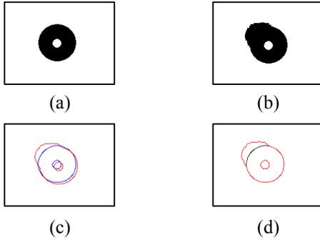
Figure 1. E-M position on circular fiducials in PCB (a) template (b) test fiducial; (c) alignment with equal weights (initial solution); (d) E-M alignment result.
