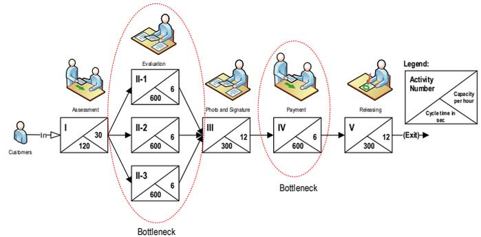
Figure 7. Diagram of Service Line Bottleneck
