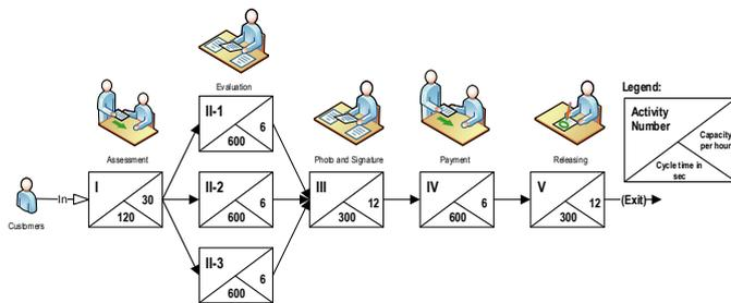
Figure 6. Process Flow Diagram with Cycle Time and Capacity
