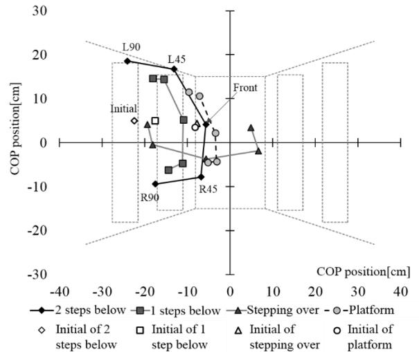
Figure 8: Horizontal coordinates of COP during initial posture and maximum reach. Colorless markers express values during maximum reach. Colored markers are connected in order as follows: Left-90°, Left-45°, Forward, Right-45°, Right-90°. Dotted lines express the outer shape of the stepladder.
