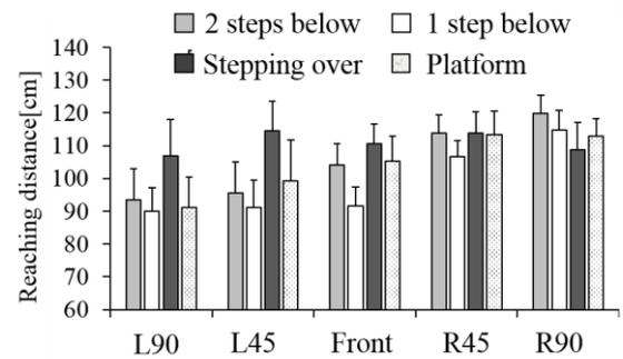
Figure 6: Horizontal reach distance from the center of the stepladder to the fingertip.
