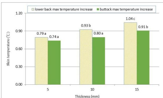
Figure 8: The thickness effect on maximum skin temperature increase (a, b: Duncan grouping code), mean.
