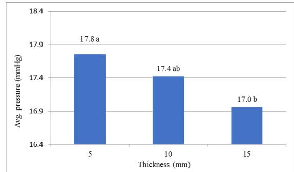
Figure 4: The thickness effect on average pressure (a, b: Duncan grouping code), mean.
