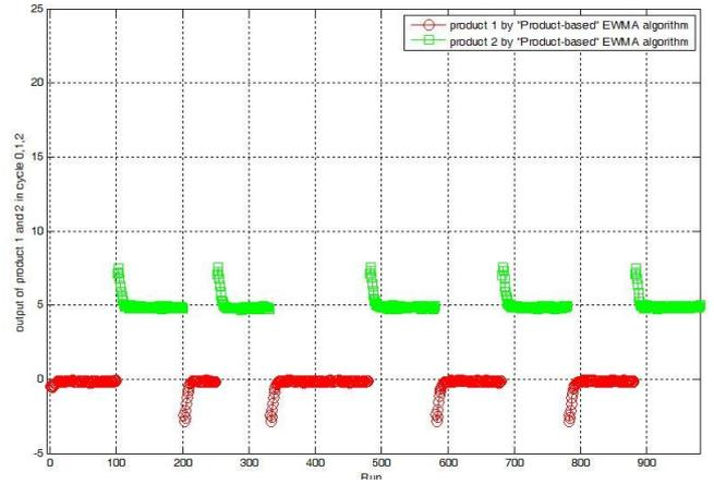
Figure 4. Controlled outputs of the tool-based EWMA control for Products 1 and 2.
