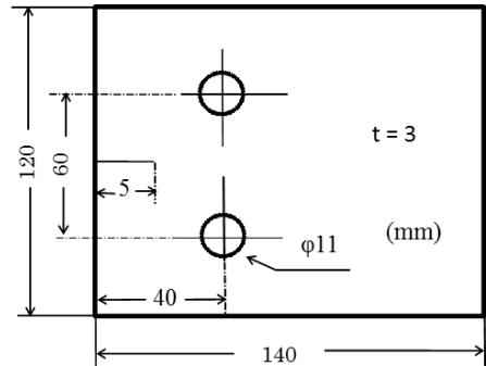
Figure 3: Geometry of the specimen
