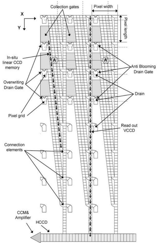
Figure 1: Plane structure of the image sensor with a slanted linear CCD memory in each pixel
