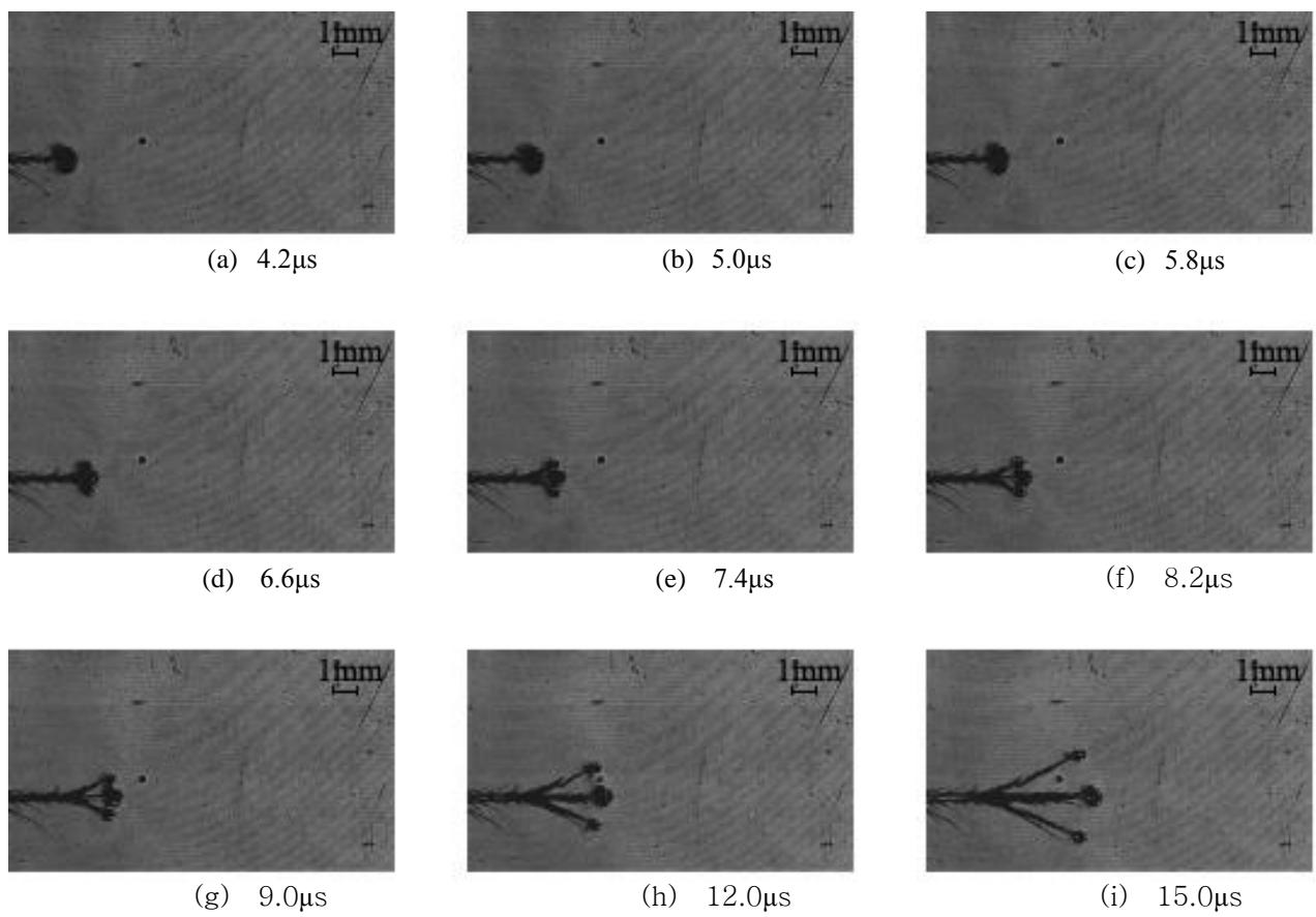
Figure 5: Bifurcation captured with the frame rate
