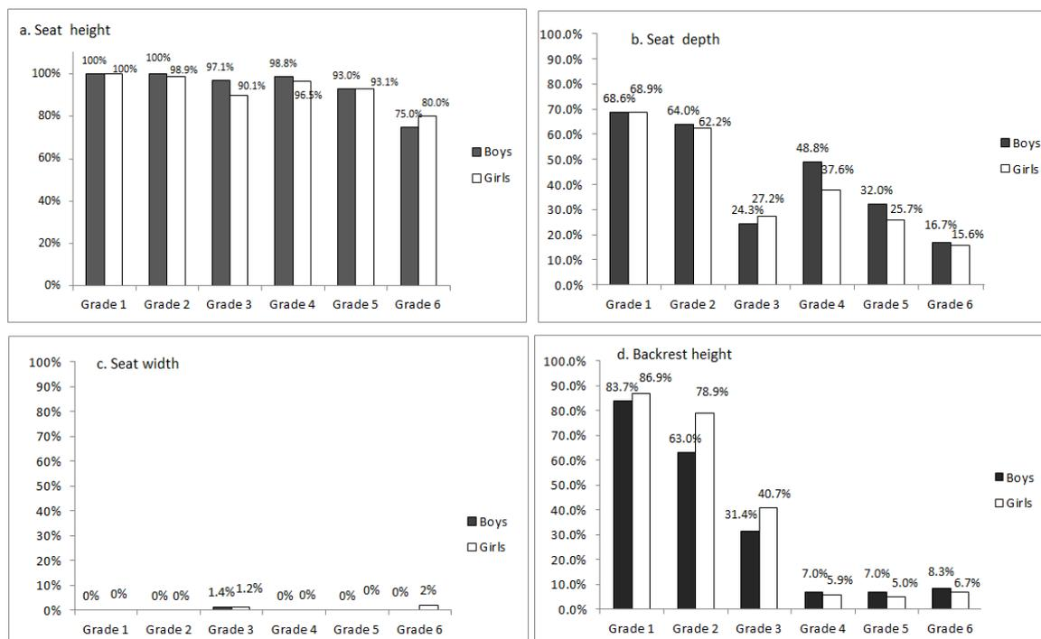
Figure 3. The mismatch percentages for seat dimensions by gender and grade level
