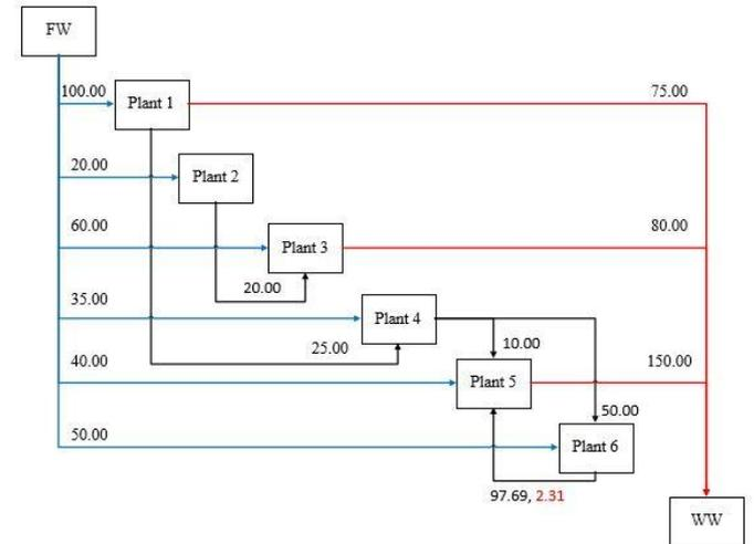
Figure 6: Optimal EIP Network without Resiliency
