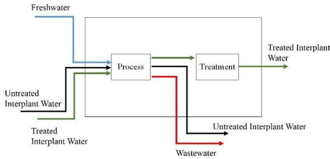
Figure 2: Possible Input and Output Water Flowrates in a Plant
