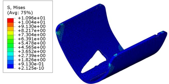
**Figure 9: FEA Results for Limb Attachment (After Optimization)**
