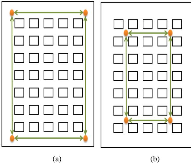
Figure 2: The illustration of the (a) outer design and (b) inner design of register marks.
