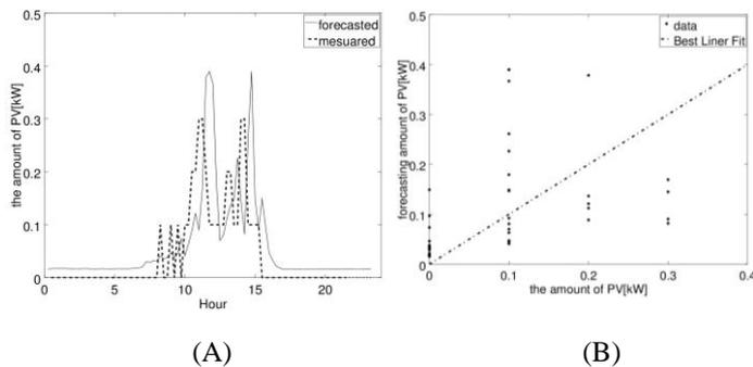
Figure7: Forecasted PV generation after 30 minutes on 2014/10/5.
