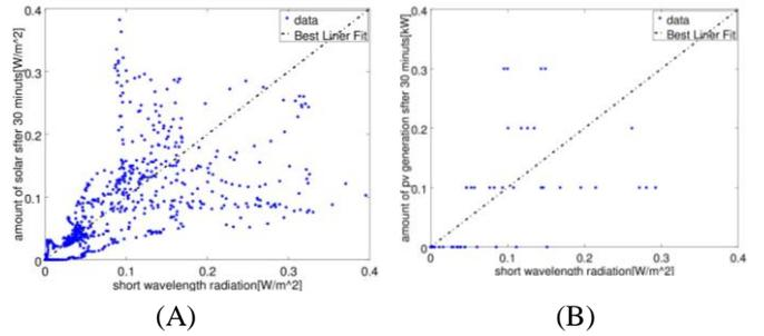
Figure3: Correlation diagram between short wavelength radiation and PV.
