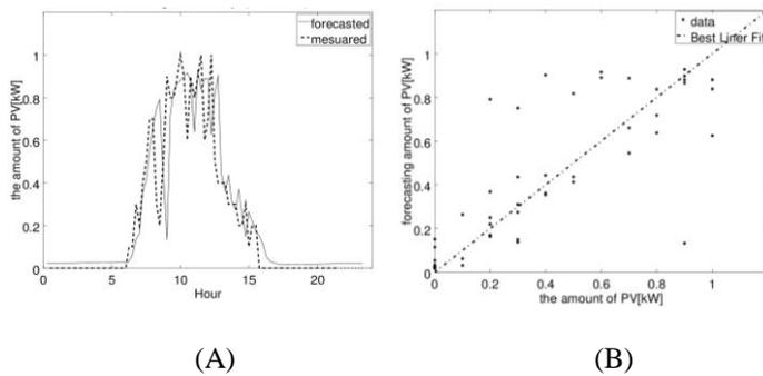
Figure11: Forecast PV generation after 30 minutes on 2014/10/15.
