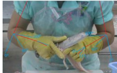
Figure 6: Motion 5, Remove excess parts near the top of the fish fillet
