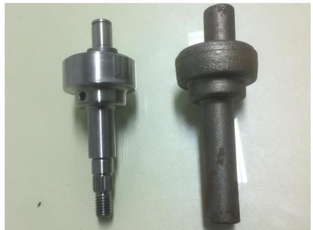
Figure 3: Product photos (cold forging, hot forging).
