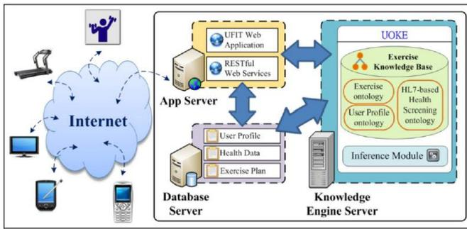
Figure 3 MIFIT physical architecture
