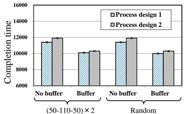
Figure 7: Simulation results for productivity of both designed lines
