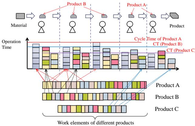
Figure 2: Schematic diagram for design of process line by line balancing each product for mixed production line
