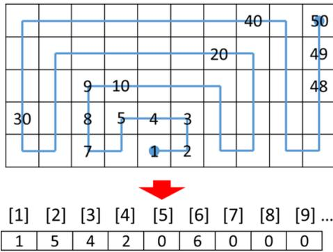
Figure 9: Chromosome representation and relationship between cells and chromosome elements
