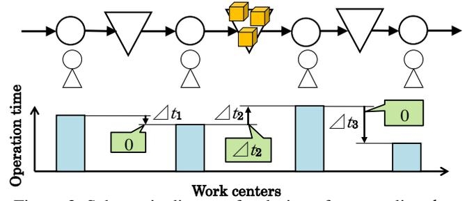
Figure 3: Schematic diagram for design of process line that includes assignment of jobs for reducing inventory between work centers
