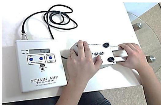
Figure 3: Grip strength for handbrake measured by handbrake dynamometer
