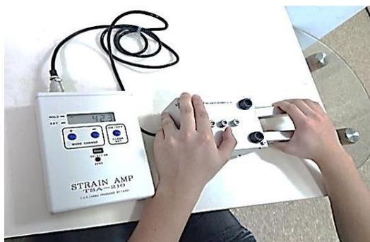
Figure 3: Grip strength for handbrake measured by handbrake dynamometer
