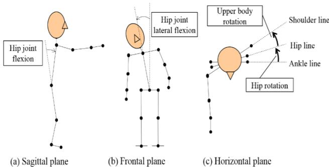
Figure 4: Definition of joint angles.
