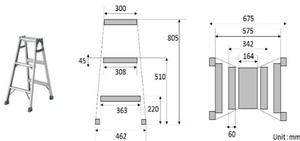
Figure 1: Dimensions of the stepladder used in this experiment. A photo, the side view, and the top view.
