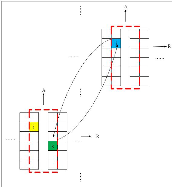
Figure 3: Exchange locations between different R-A area
